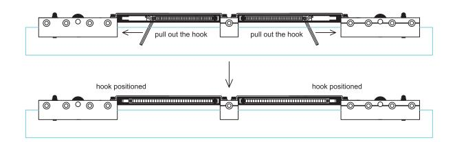
B: Please notice that the damping device can be push inward or outward to be closer to the active device when you release the hex head screw.
